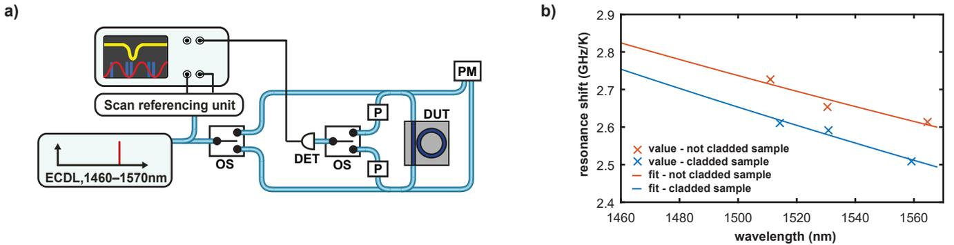
**Fig. S1.** a) Setup used to record resonance skewing upon driving laser power increase. OS: optical switch, DET: photodetector, PM: power meter, DUT: device under test, P: polarizer. b) Resonance shift upon constant heating characterized for cladded and non-cladded samples, as well as fit with a linear function.
