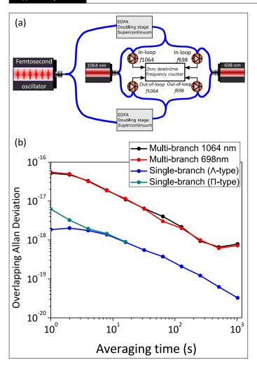
**Fig. S1.** (a) Experimental setup used to characterize the visible optical frequency comb generation in dual- and single-branch configuration. EDFA: erbium doped optical amplifier. (b) Out-of-loop fractional frequency instability of the 698 nm and 1064 nm beatnote with the visible comb in dual-branch configuration (red and black curve) and the frequency ratio (blue and green curve,  $\Lambda$  and  $\Pi$ , respectively).
