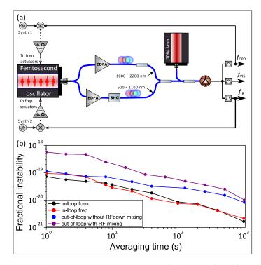
**Fig. S3.** (Experimental setup to estimate the limits induced by the electrical detection and processing of the coherent stitching of the two supercontinua. (b) Fractional instability in terms of Allan deviation of the in-loop servo locking errors of  $f_{ceo}$  and  $f_{rep}$ ), the out-of-loop measurement with RF down mixing (purple curve) and without RF down mixing (blue curve). See text for details.
