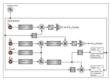
**Fig. S2.** Setup of the electrical detection and processing of the optical beatnote comprising the generation of error signals, and the noise characterization of the out-of-loop beatnote.
