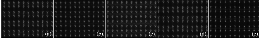
Figure. S3. Optical images of an array of the number “4” observed through PVC gels MLAs prepared by evaporation of THF from 100 \mu L PVC gels solution under different voltages: (a) V = 10 V, (b) V = 20 V, (c) V = 40 V, (d) V = 40 V and (e) V = 50 V.
