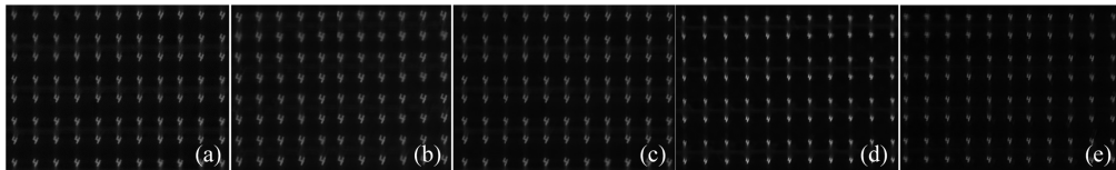
Figure. S5. Optical images of an array of number “4” observed through PVC gels-based MLAs prepared by evaporation of THF under 50 V DC field with different volumes of PVC gels solution: (a) 60 \mu L, (b) 80 \mu L, (c) 100 \mu L, (d) 120 \mu L and (e) 140 \mu L.
