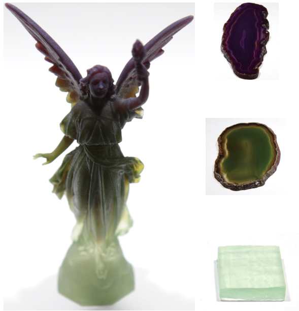
Fig. S4. The St. Lucy model printed (10cm) with varying RGBA values. At the top is that of the violet stone, middle is green stone and bottom is green soap, with linear transitions in between. Fig. reproduced from Brunton et al. [1].
