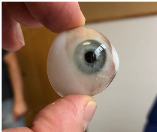
Fig. S7. 3D printed partly-textured eye prosthesis that was polished in a post-process.
