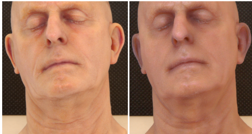
Fig. S5. 10cm head model printed with \alpha = 0.786 (left) and \alpha = 0.518 (right). Identical model geometry and illumination conditions. Fig. reproduced from Brunton et al. [1].
