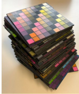
Fig. S3. Printed target used to fit the five grid point cellular Neugebauer model to predict both color and the translucency parameter \alpha [2]
