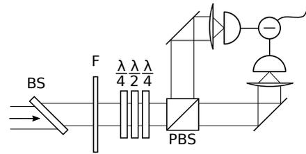
**Fig. S3.** Detail of the detection setup for one of the  $s_{1,2,3}$  Stokes parameters. See text for description.
