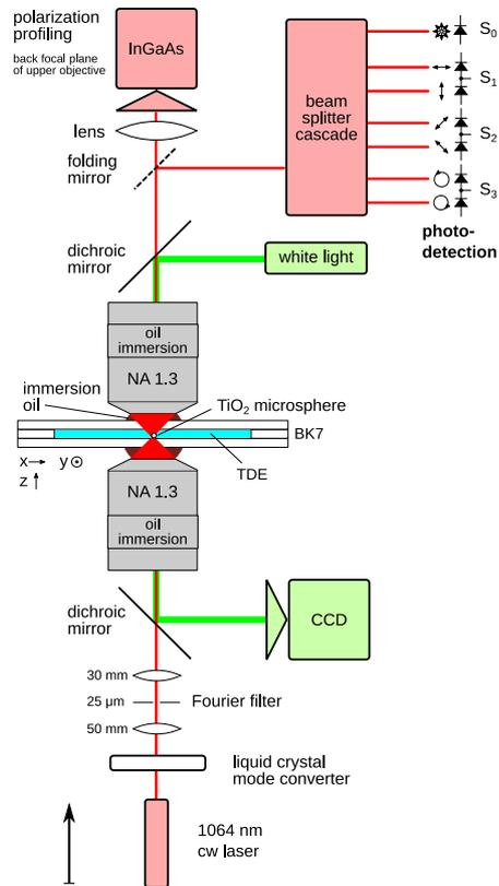
**Fig. S1.** Overview of experimental setup.
