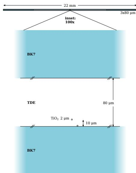
**Fig. S2.** Sample configuration (to scale).
